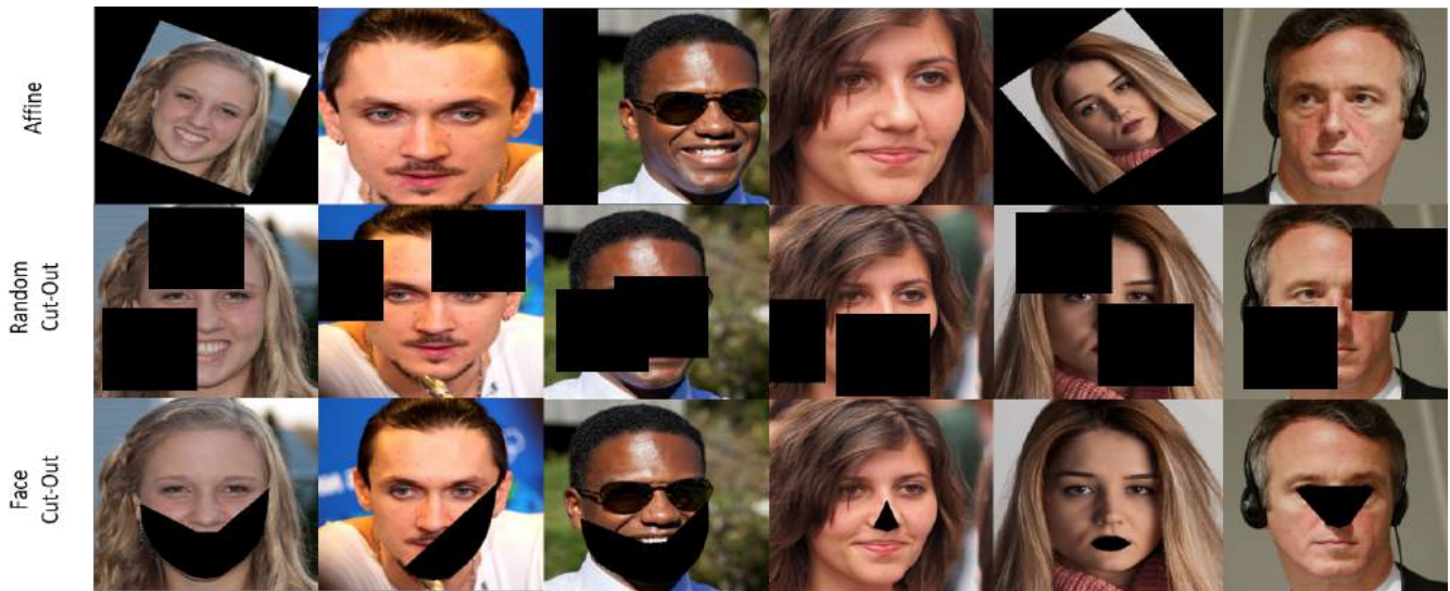
Figure 1: Our face pre-processing module is responsible for applying 3 different types of image augmentations, (1) Affine Transformations, (2) Random cut-out augmentations, and (3) Face cut-out augmentations. More details about the augmentations we use are given in upcoming sections. We show that the employed image augmentations improve detection performance while reducing overfitting. Photos acquired from Flickr Faces HQ dataset [15].
