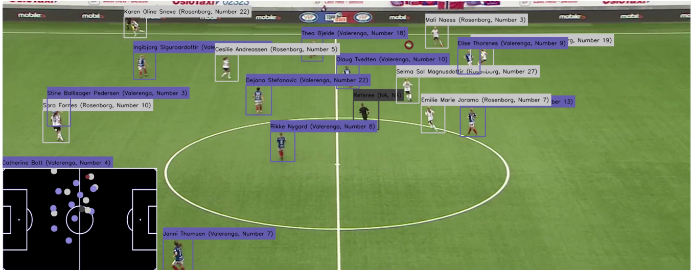
Figure 1: FootyVision multi-object tracking and top-down localisation in viewpoints with limited visual information.
